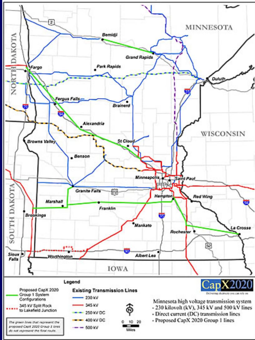
Current and Proposed High Voltage Transmission Lines
