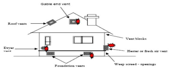
Prevent penetration from direct flame impingement Prevent penetration from firebrand exposure
