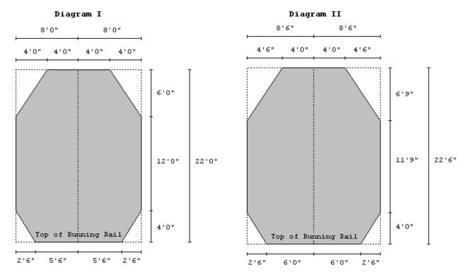
(a) Diagram I is described as follows: starting at the center line of track at top of rail and extending 5'6" both sides horizontally and level therewith, thence upward diagonally to a point 4'0" above top of rail and 8'0" laterally from center line of track, thence vertically to a point 16'0" above top of rail, thence diagonally upward to a point 22'0" above top of rail and 4'0" horizontally from center of track, thence horizontally to center of track.
